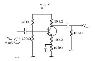
The output voltage, V<sub>out</sub> is nearly:
