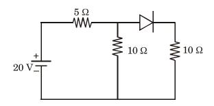
The minimum power rating of the diode should be:
