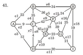
V = {A, B, C, D, E, F, G, H, I} E = {e1 = (A, B), e2 = (A, C), e3 = (A, D), e4 = (B, C), e5 = (B, F), e6 = (B, H), e7 = (C, D), e8 = (C, E), e9 = (C, F), e10 = (D, E), e11 = (D, I), e12 = (E, F), e13 = (E, G), e14 = (F, G), e15 = (F, H), e16 = (G, H), e17 = (G, I), e18 = (H, I)}
