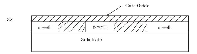
Gate oxide layer consists of :
