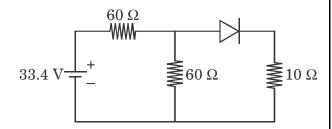
If the voltage drop across the diode is 0.7 Volt, then the diode used should have minimum power rating nearly:
